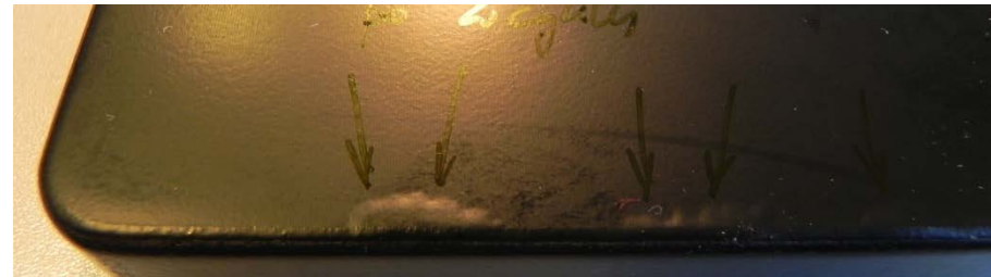
A-I-15 after 5 cycles, swelling of the coating along the whole edge
